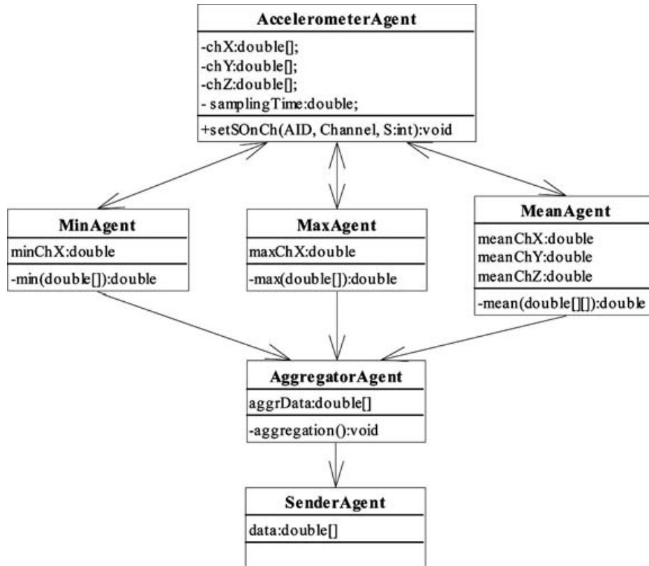
Figure 5.6. ASPINE-based design of the example in-node signal processing task.
