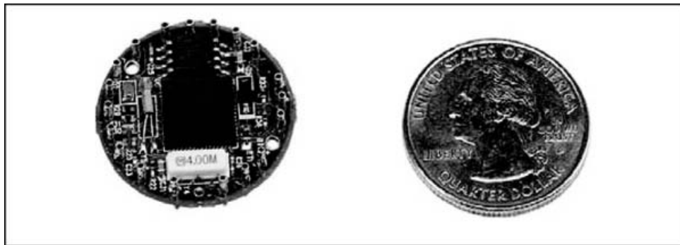
Figure 6.6. A Mica2DOT board (taken from www.xbow.com ). See also Color Insert.
