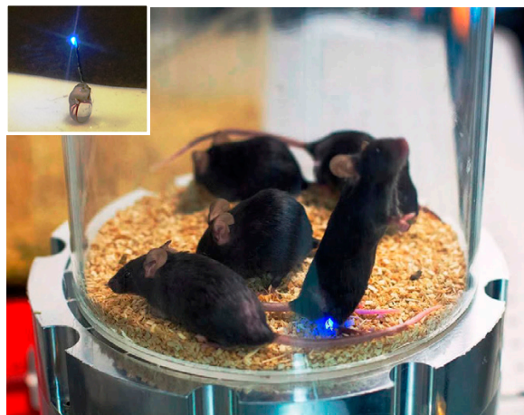
A resonant cavity (top) powers the wireless optogenetic platform developed by Ada Poon and colleagues at Stanford, using commercially available components. Wirelessly powered internal implants (inset, bottom) enable the mouse to move freely and behave normally while receiving optogenetic stimulation of peripheral nerve endings in the hind paw. A. Poon/Stanford University
