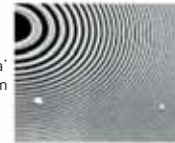
Zone plate x-ray 'Lena' outer ring spaces ~35 nm
