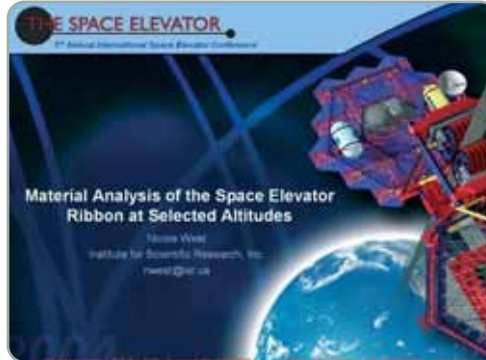
Space elevator project (USA): Goal is to develop a 60% CNT filled polymer (PMMA or PS) with an exceptional tensile strength of 60 GPa. Current status for these composites is 2-4 GPa Existing high strength fibers such as carbon fiber, aramide, dyneema, PBO are in the range of 3-6 GPa.
