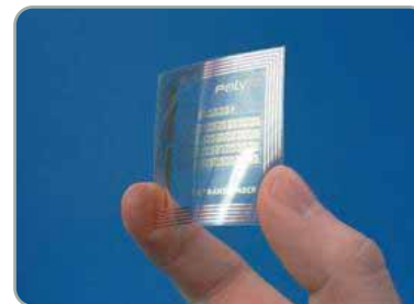
Polymer 13.56 MHz RFID tag of PolyIC
