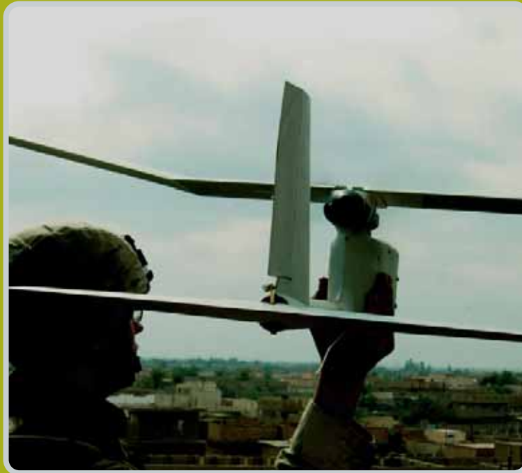
Future now: soldier launches a Raven “Unmanned Aerial Vehicle” (UAV) to conduct reconnaissance for insurgents in Iraq (Photo US DoD)
